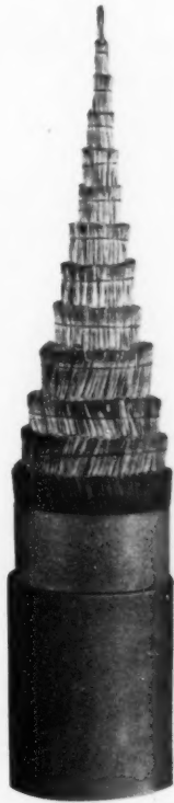
Fig. 4—Typical construction of long distance telephone cable.
